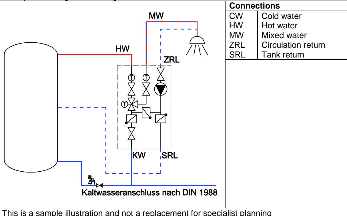
Example: combined buffer storage with internal drinking water heat exchanger
