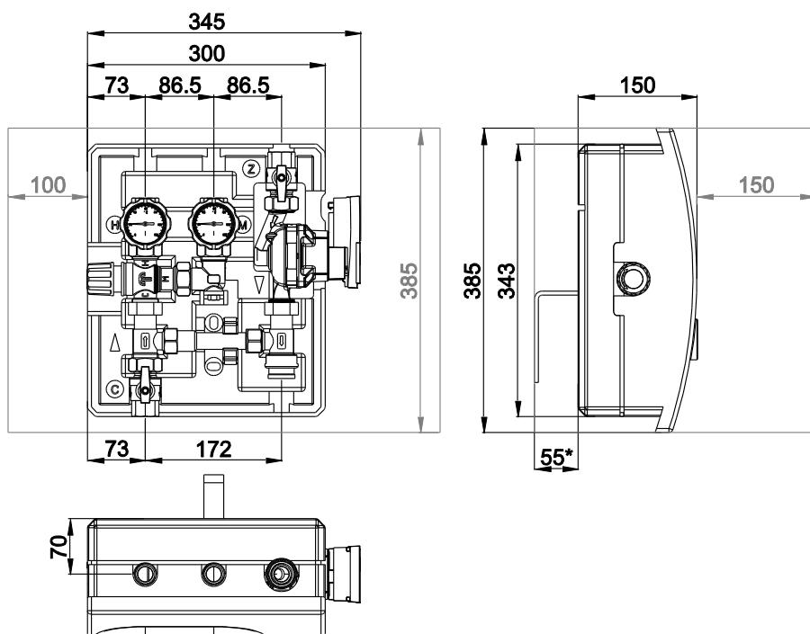
\* Installation flush with walls possible
